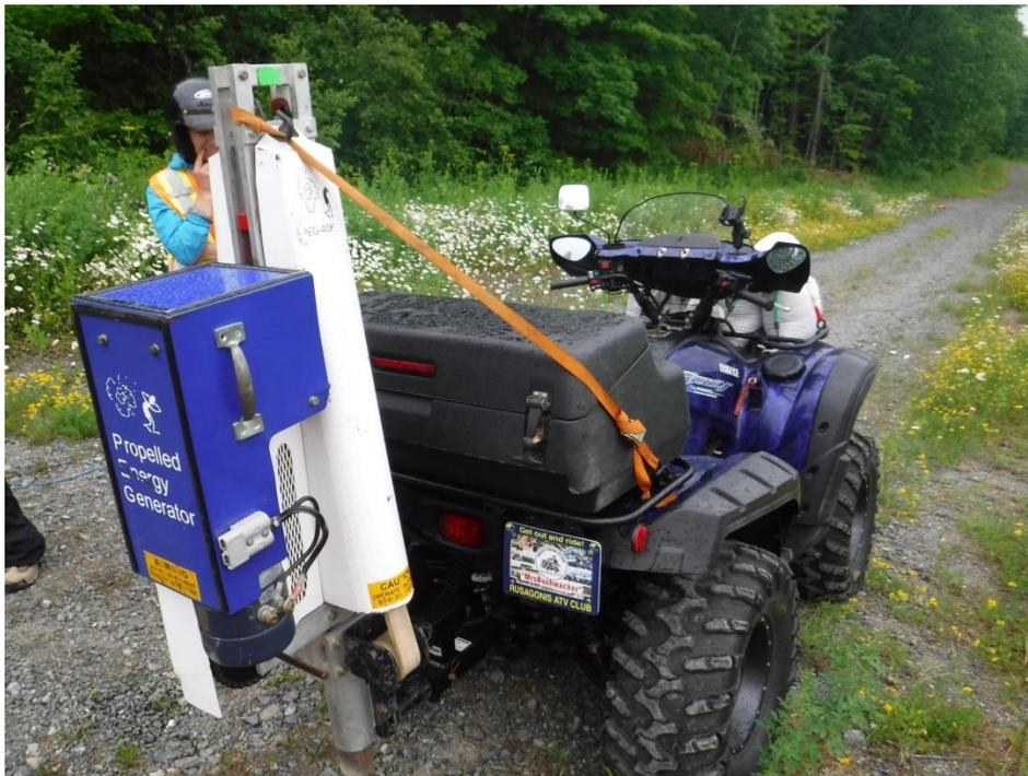
Above: Impact testing device (Propelled energy generator)
