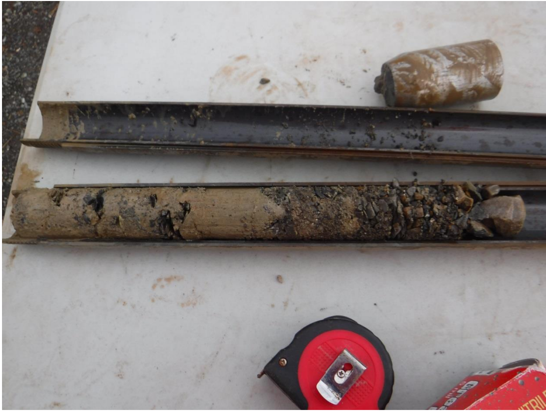
Above: A core tube composed of loose fill and glacial till.
